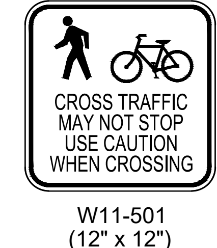
W11-501 (12" x 12") PEDESTRIAN SYMBOL HEIGHT - 4" (IN) BICYCLE SYMBOL HEIGHT - 3" (IN) LETTERS - 1" C LEGEND - BLACK BACKGROUND - YELLOW
